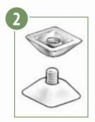
Pyranut #2 is installed as shown, so it's a half turn away from #1.
